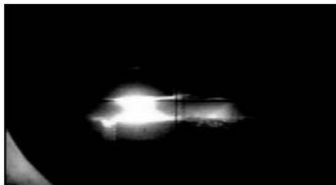
Figure 2.22 Photograph of an arc looking as a braid
